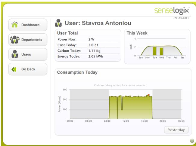
Figure 1 - Meter to User Level Energy Dashboard
